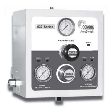
The 637 Series AutoSwitch system permits a high pressure reserve for a primary liquid cylinder or bank of liquid cylinders. Visible alarms on the enclosure or an optional remote alarm signal the need to replenish the liquid cylinder.
